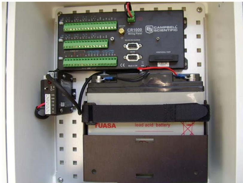
Figure 2(b) CH100 charger mounted alongside a BP17 in a typical logger-enclosure configuration
