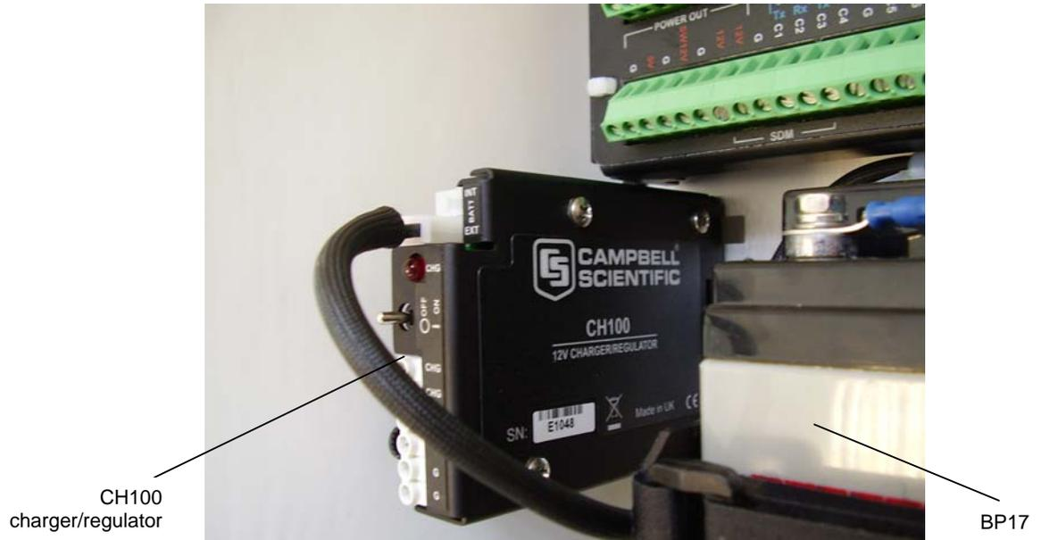
Figure 2(a) CH100 charger mounted alongside a BP17 in a typical logger-enclosure configuration
